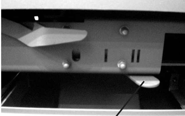
Operating lever for combustion air supply
